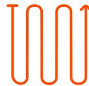
Neato uses LaserSmart technology to plan the most efficient course and clean in record time. Because it's not wasting energy bouncing around like round robots, it can clean more space on a single charge. If it needs more power, it automatically returns to the charge base, powers up, then goes back to finish the job.
